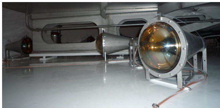
Figure 2.10: Hamamatsu R1408 8" PMT in the IV, encapsulated in stainless steel.
