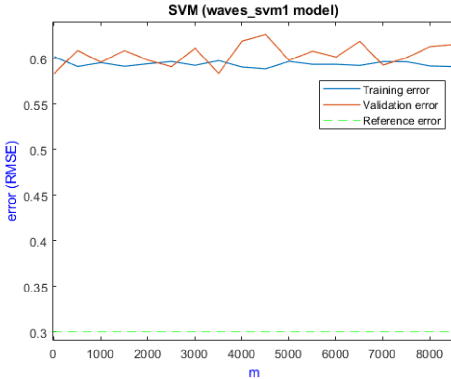
Figure 8.3. Learning curves plot for waves_svm1 model trained with data from 2018 and using 5-fold Cross Validation scheme
