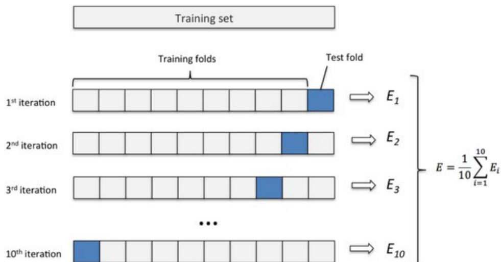
Figure 3.11. Diagram of k -fold cross-validation algorithm represented for k = 10 . Image obtained from http://karlrosaen.com/ml/learning-log/2016-06-20/
