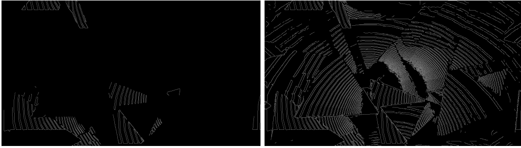
(a) Canny output with wrong threshold values (b) Canny output with best threshold values
