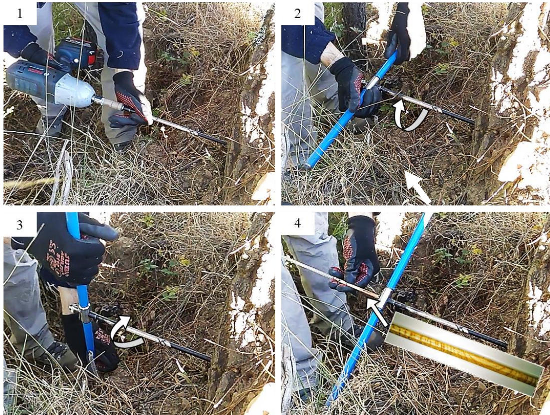
Fig. 12. Example of core extraction with the help of an increment borer of the Pressler type. (1) Detail of the power drill at the borer insertion point, (2) and (3) a mini-auger is drilled by hand from the bark to the centre (pith) of the tree, and (4) the resulting core sample extracted from the hole, which displays the tree's annual rings at that point in the tree. Pictures by ©Callejas-Díaz, M., 2018.
