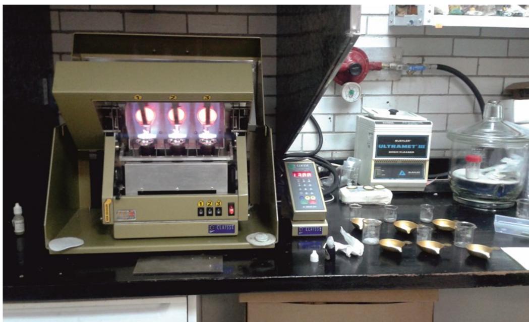
Fig. 3.5 Oven melting three pulverized rock samples on the left and six other samples on their platinum fuse vessels already mixed with 25% LiBr solution (small black bottle) on the right.
