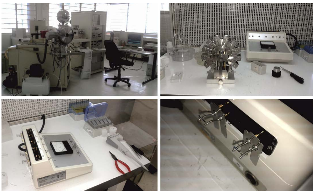
Fig. 3.8 From top left to bottom right photographs: Finnigan MAT262 Thermal Ionization Mass Spectrometer (TIMS) used to analyse the lead samples; cartridge to insert the samples in the source chamber of the mass spectrometer; voltmeter to load the samples on the filaments; and Re filaments with the samples loaded.
