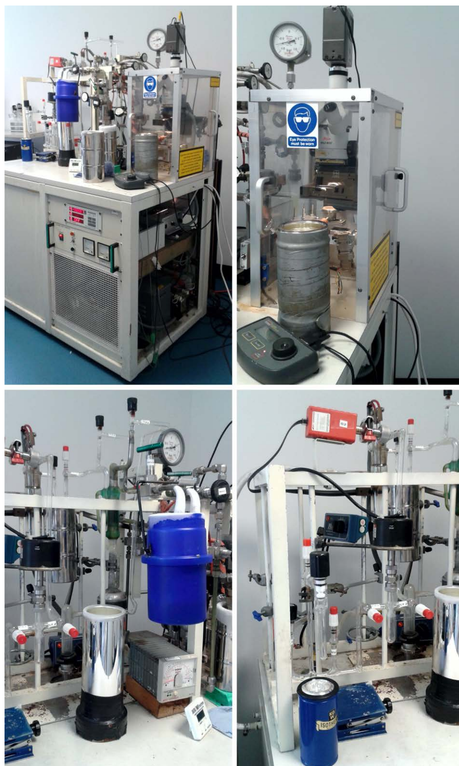
Fig. 3.8 Up left: general view of the fluorination line; Up right: Laser cage and reaction chamber; Bottom left: Pipes to conduct the molecular oxygen from the reaction chamber to the carbon rod in order to transform it into CO 2 ; Bottom right: cold finger and sample tube for the mass spectrometer.
