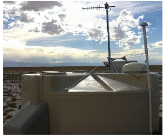
(b) EASIER antenna mounted on an SD detector
