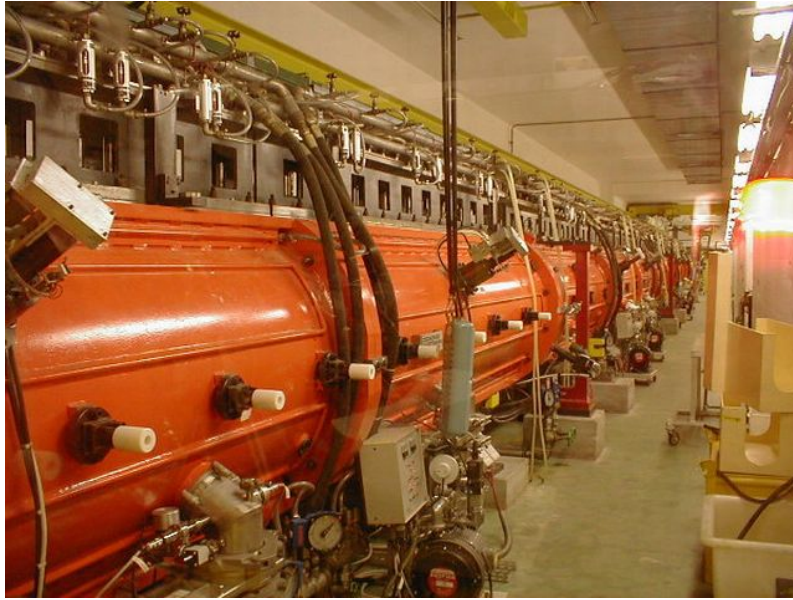
Figure 3.1: Picture of the Linac-2 acceleration tanks, which accelerate the protons to inject them into the PS-Booster.
