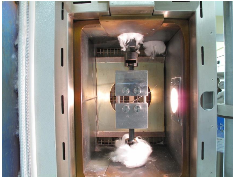
Fig. 2.3.2. A sample in the furnace of the Instron machine. The thermocouple wires are attached to the gauge section of the sample.
