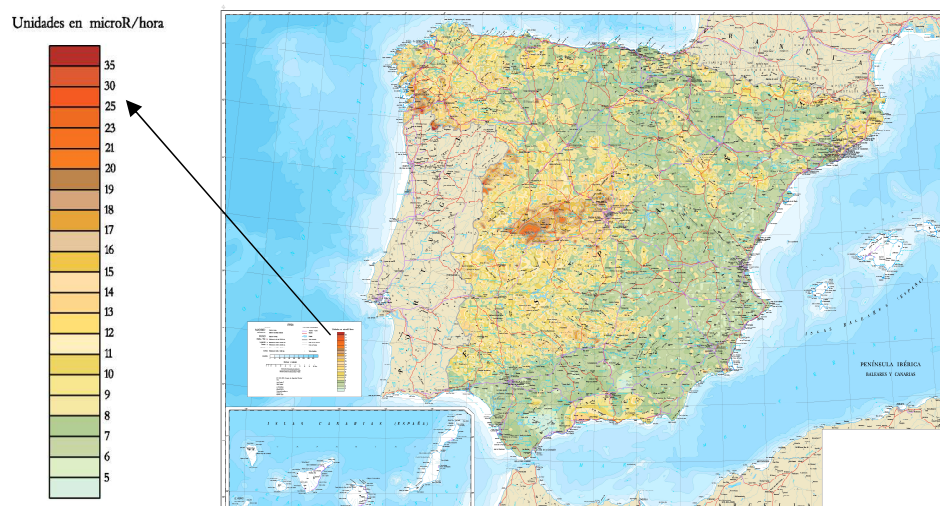
Figure 8. Map of the natural gamma radiation ( \mu\text{R}/\text{h} ) 49 in Spain. Scale 1/1000000. (MARNA Project) 50 .
