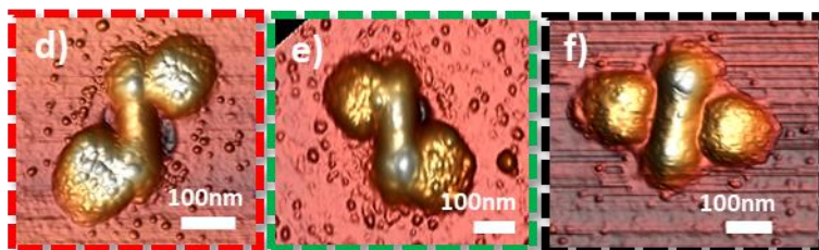
Figure 8.3.3 AFM images of nanohybrid structures with gold disk dimers (a-c) and dielectric disk dimers of \text{CaF}_2 (d-f). For both structures the nanorods are made of multilayers with cobalt and gold and the dimers are at 45^\circ (a-d), -45^\circ (b-e) and 90^\circ (c-f).
