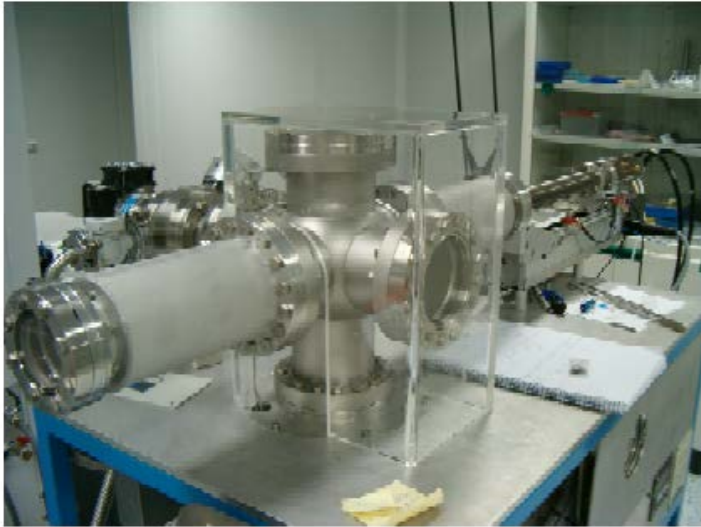
Figure 3.2. View of the sputtering chamber. The targets are mounted on a remote controlled arm to switch between the different materials.
