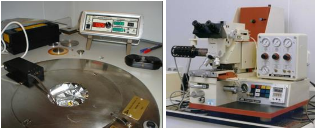
Figure II.8: Image of the Headway Research spinner (in the left hand side) and the MJB3 UV400 alignment system (in the right hand side), used for the lithography process.
