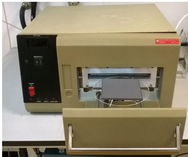
Figure II.9: Image of the RTA system.
