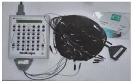
Figure 4 NeuorScan 4.5 acquisition system
