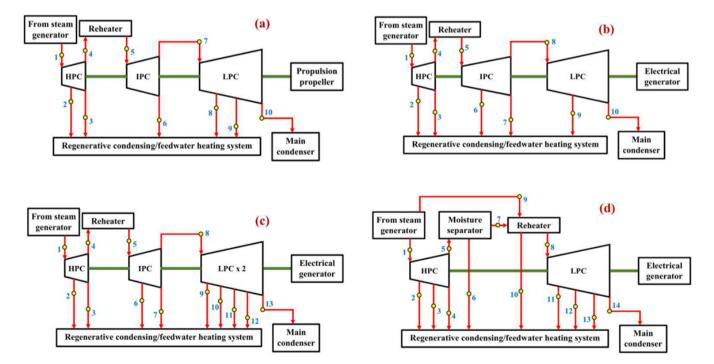
Fig. 1 General schemes of the observed steam turbines along with operating points required for the analysis:(a) Marine propulsion steam turbine;(b) Steam turbine from the conventional power plant;(c) Steam turbine from ultra-supercritical power plant;(d) Steam turbine from nuclear power plant
