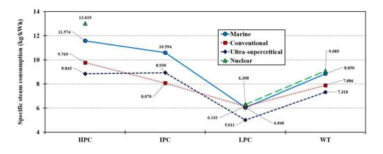
Fig. 9 Specific steam consumption of each cylinder and whole turbine
