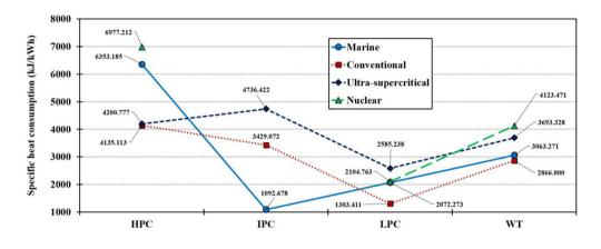
Fig. 10 Specific heat consumption of each cylinder and whole turbine
