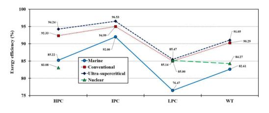
Fig. 8 Exergy efficiency of each cylinder and whole turbine
