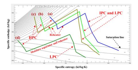
Fig. 2 Steam expansion and reheating process in *h-s* diagram through all cylinders of all analyzed steam turbines:
