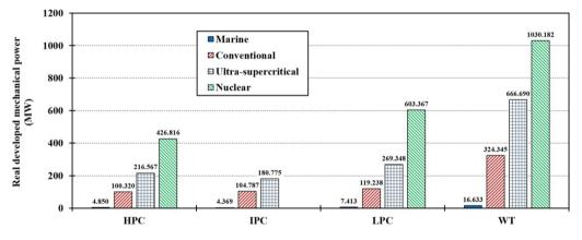
Fig. 4 Real developed mechanical power of each cylinder and whole turbine
