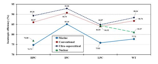
Fig. 6 Isentropic efficiency of each cylinder and whole turbine
