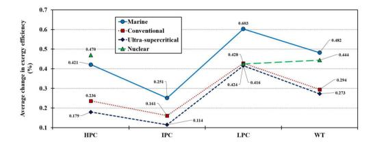
Fig. 11 Average change in exergy efficiency (between ambient temperatures 5 °C and 45 °C) of each cylinder and whole turbine
