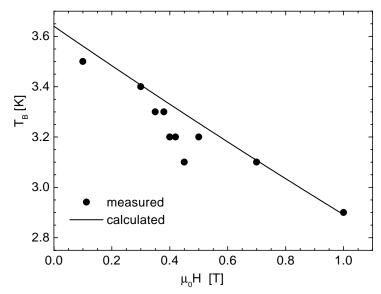
Fig. 2. Measured and calculated dependence of blocking temperature  $T_{\rm B}$  on applied magnetic field H.
