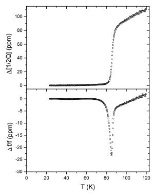
Fig. 1. Zero field temperature dependence of the imaginary and real parts of the complex frequency shift  $\frac{\Delta\widetilde{\omega}}{\omega} = \frac{\Delta f}{f} + \mathrm{i}\Delta\left(\frac{1}{2Q}\right)$  for a thin film YBa<sub>2</sub>Cu<sub>3</sub>O<sub>7- $\delta$ </sub> on MgO substrate.
