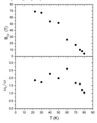
Fig. 4. The upper critical field  $B_{c_2}(T)$  and the ratio of the depinning frequency  $\omega_0(T)$  to the measurement frequency  $\omega = 2\pi \times 9.28$  GHz, obtained as the best fit parameters for the curves in Fig. 3.
