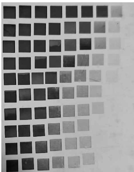
Figure 2 Laser marking samples
