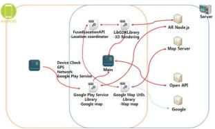
Figure 5 Overall system configuration
