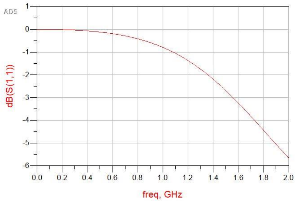
Figure 5.9: Tunable filter frequency response with a 1V tuning voltage
