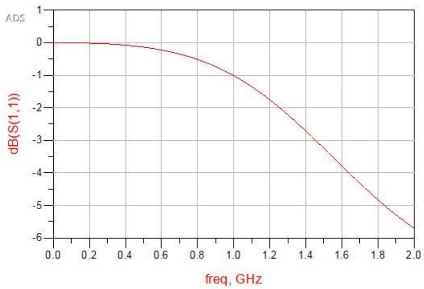
Figure 5.10: Tunable filter frequency response with a 5V tuning voltage
