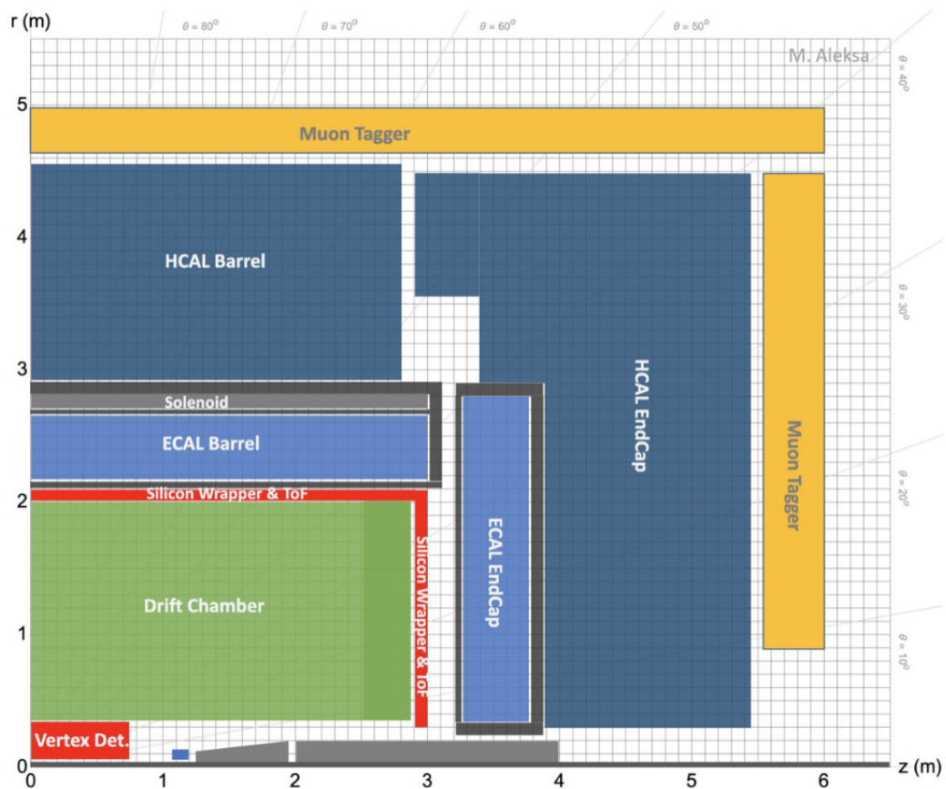
Figure 2.4: Detector concept for the FCC-ee with a LAr calorimeter [12]
