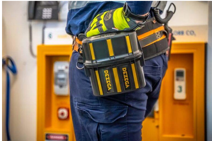
Figure 6 Self-Contained Self-Rescuer - DEZEGA Ci-30 KS. Credit: MineARC Systems.
