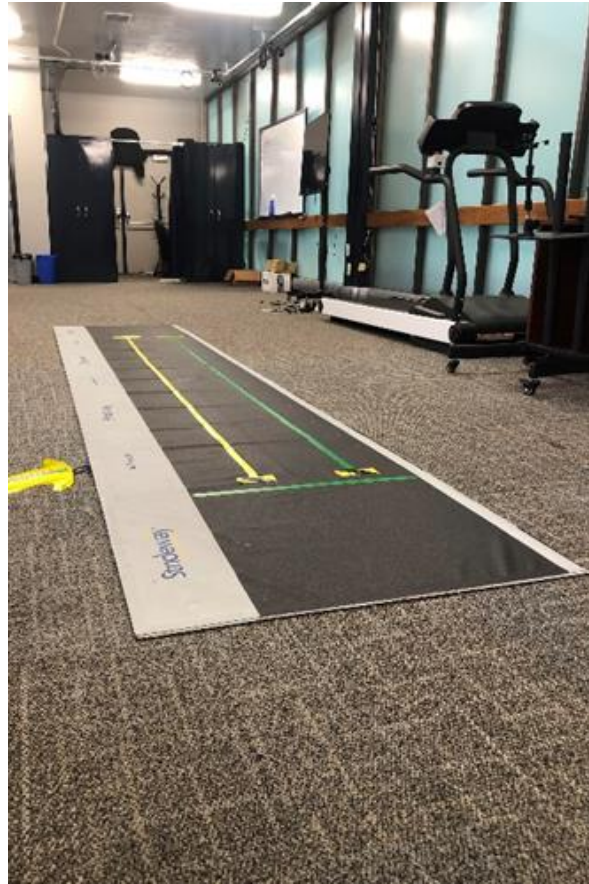
Figure 3. Teckscan Strideway (30 Hz, Tekscan Inc., South Boston, MA) that will be used to record all trials.
