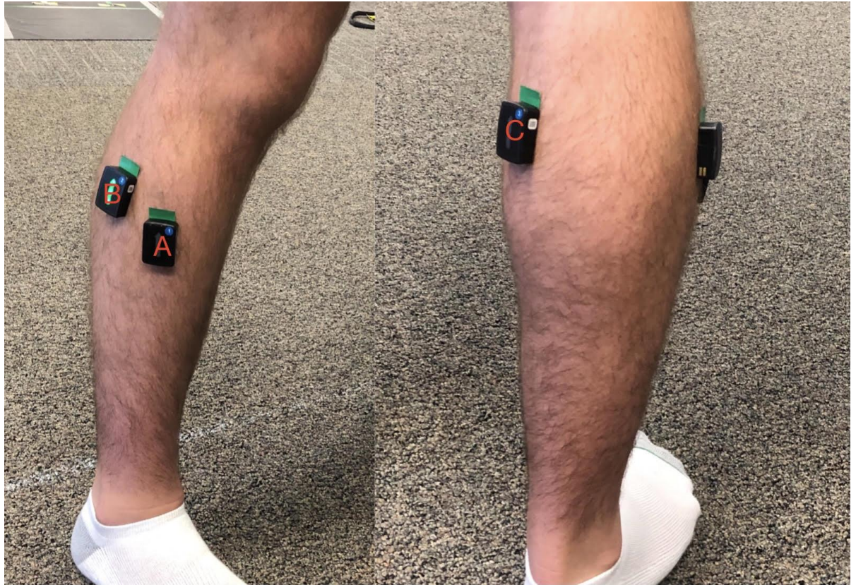
Figure 2. Delsys sEMG Electrodes (2000 Hz, Delsys, Natick, MA) on the Tibialis Anterior, Peroneal, and Medial Gastrocnemius
