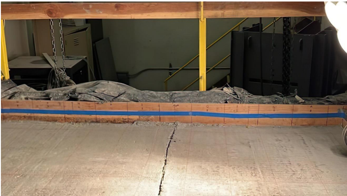
Figure 13. PCC Slab After Applying Aging Procedure.
