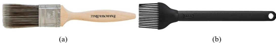
Figure 14. (a) Paint Brush used for Emulsified Asphalt Application, (b) Silicone Brush used for Hot-Applied Asphalt Binder Application.
