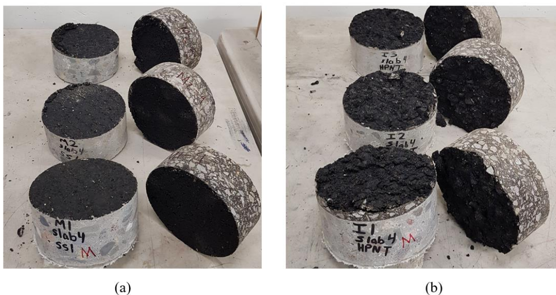
Figure 44. (a) New AC (½ inch NMAS)/Aged PCC Adhesive Failure (SS-1); (b) New AC (½ inch NMAS)/Aged PCC Cohesive Failure (HP NT).
