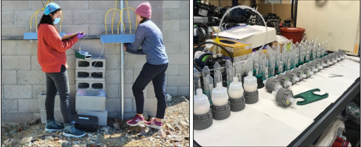
Figure 6. A general RMAS sample collection. On the left, the RMAS flow rate was being checked (at Peavine) before membrane cartridges were removed from the RMAS shield and brought inside for membrane collection. On the right was the collection process for membranes from the cartridges (at the Greenhouse). The green wrench shown was used to loosen each membrane cartridge and tweezers were used to place each membrane sample into its own conical tube, shown behind the membrane cartridges.
