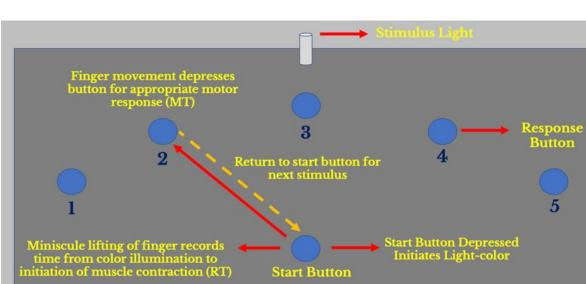
**<u>Figure-1</u>**. Configuration and sequencing of the reaction-time apparatus.
