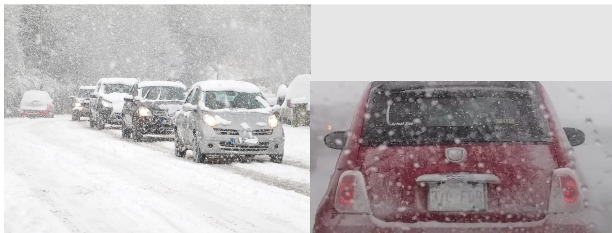
Figure 19. Heavy snow and ice prevent license plates from being detected.
