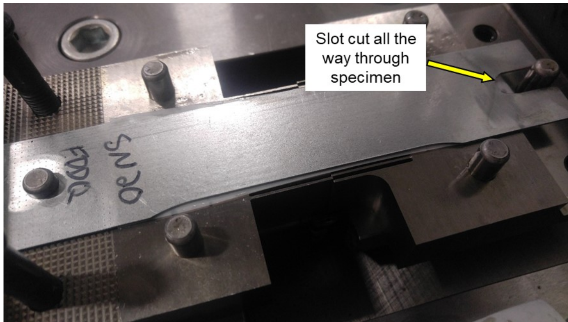
Figure 4.17: Modified CTC specimen for friction testing.
