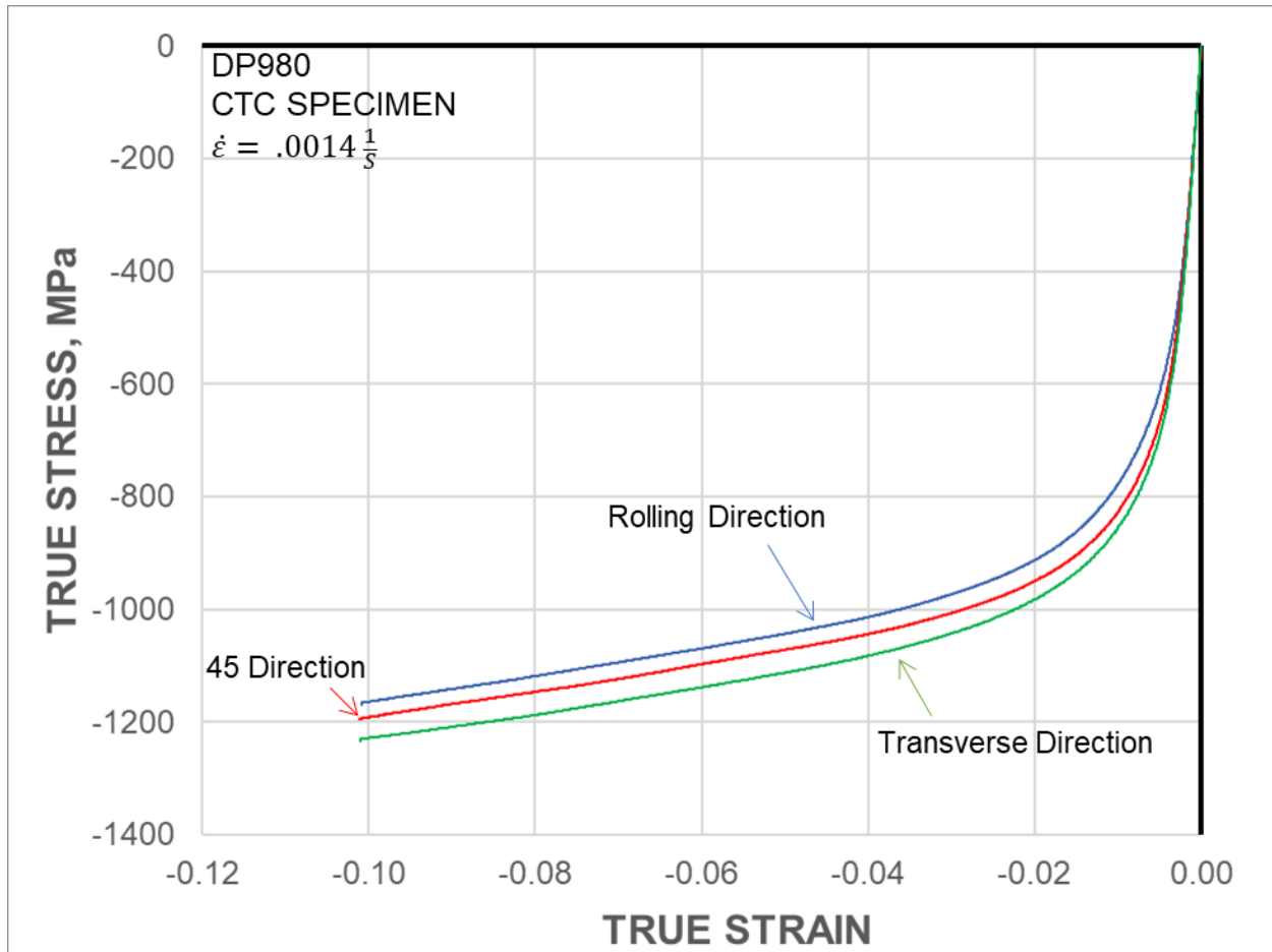
Figure 5.16 Comparing pure compression of different orientations of DP980.
