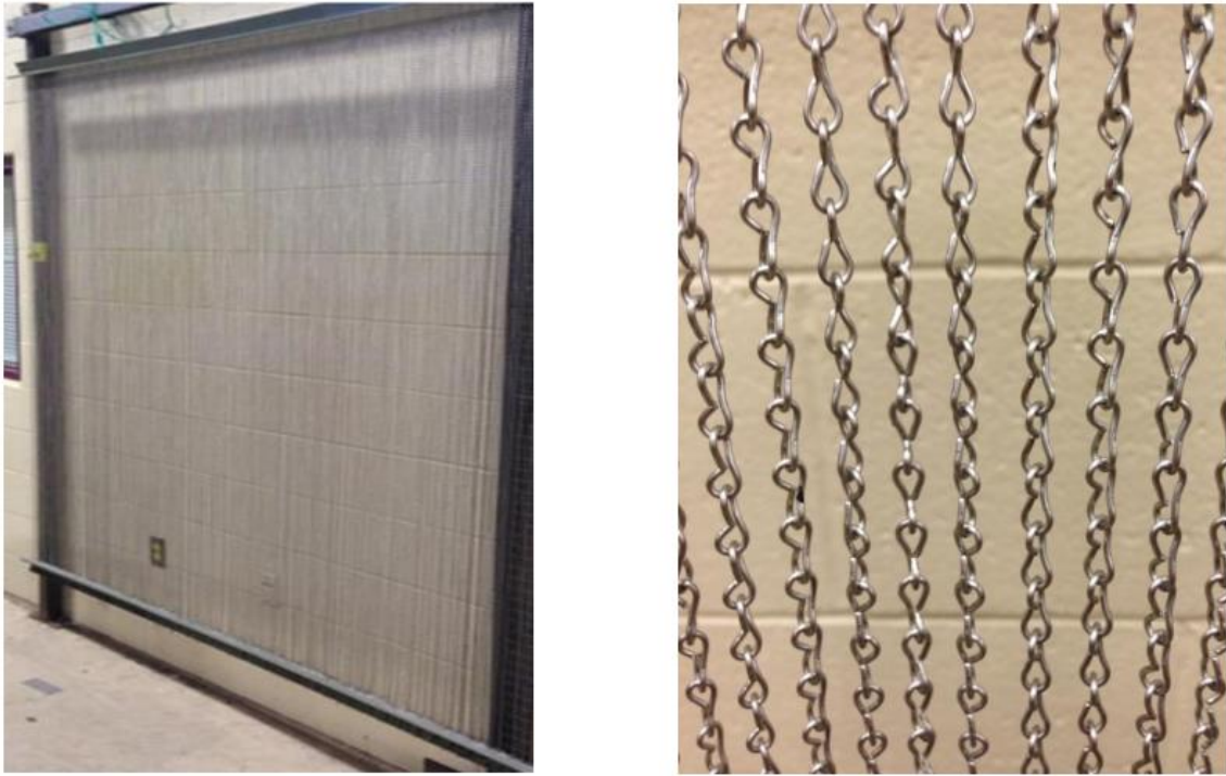
Figure 4.3: Jack-chain extended reference target: entire target (left); close up (right). From Heaton (2014).
