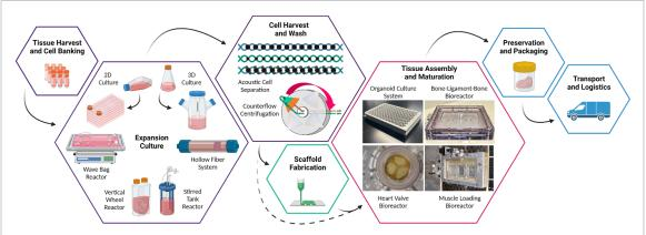
**Figure 1.** Steps of the cell and tissue manufacturing process. Many unique bioreactor form factors exist to expand cells (e.g. hollow fiber systems, stir tanks, wave bags, vertical wheels) and grow organs and tissues (e.g. bone-ligament bone (CGEM<sup>™</sup> by STEL Technologies), heart valves (Aptus Bioreactors), muscle (TEMR by George Christ at Univ. of Virginia, bioreactor by DEKA Integrated Solutions Corp), or organoids (System by Tommy Angelini)) (graphic created with BioRender.com).
