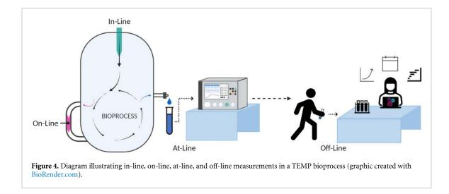
returned to the process stream [5]. An at-line measurement removes or isolates the sample to be rapidly analyzed in close proximity to the process stream [5]. This contrasts with an off-line measurement in which the sample is removed, isolated from, and analyzed in an area remote from the manufacturing process [5]. The location of the sensor or where the sample is extracted within the system will also impact how the reading is interpreted (i.e. local vs global, specific vs bulk).
