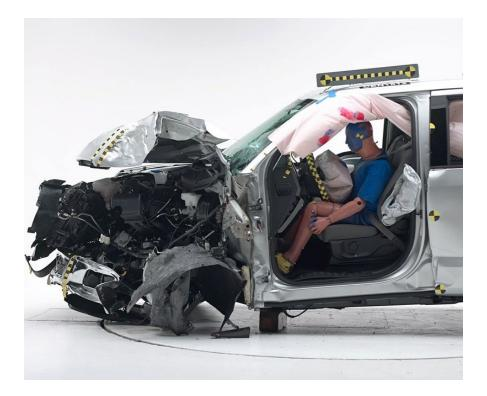
Figure 18 - 2020 Ford F-150 driver-side small overlap frontal crash test [49].
