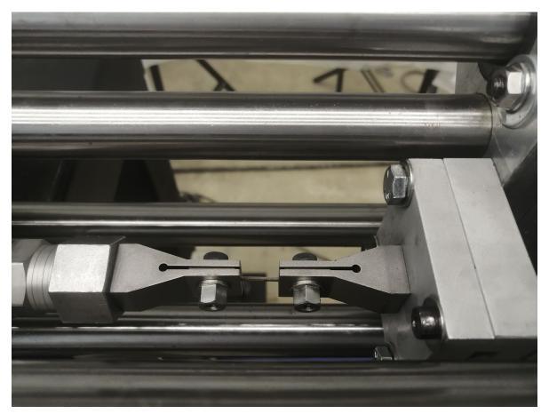
Figure 32 - Mounted IRTTA grips with mini dogbone specimen.
