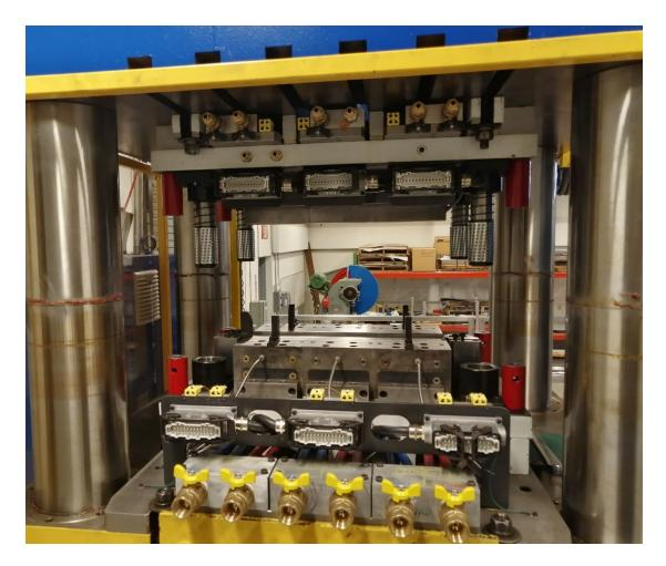
Figure 39 - Hot stamping channel die (front view).
