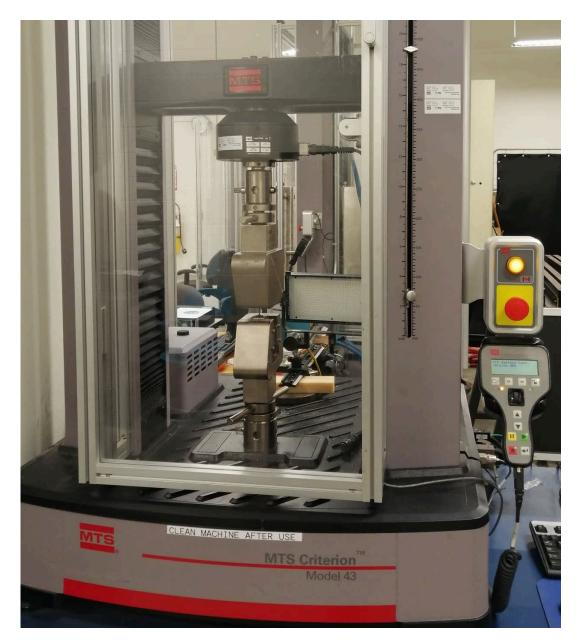
Figure 27 - MTS Criterion model 43 universal testing machine.
