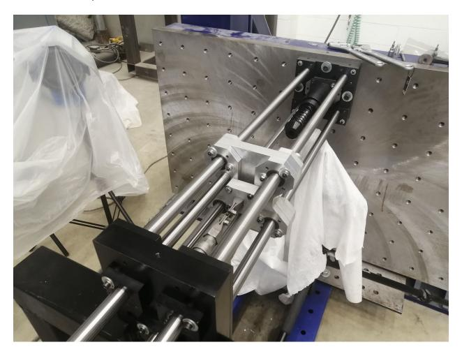
Figure 29 - Intermediate rate tensile testing apparatus with mini dogbone specimen.
