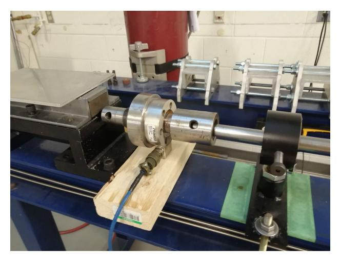
Figure 38 - Split Hopkinson bar load cell calibration.
