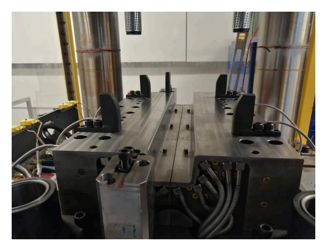
Figure 40 - Hot stamping channel die (side view).
