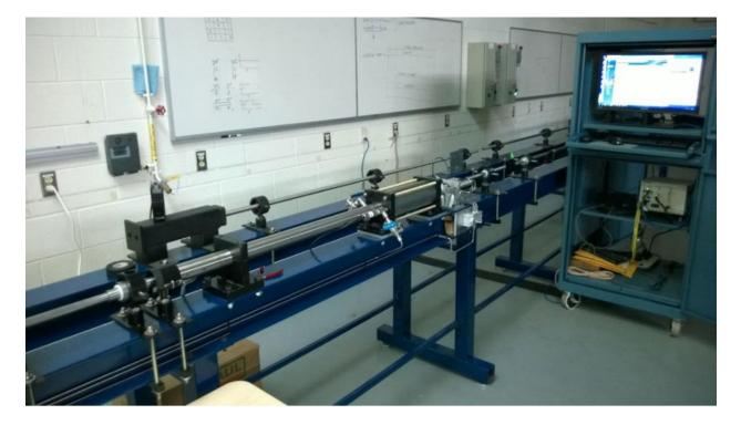
Figure 33 - Split Hopkinson pressure bar testing setup.
