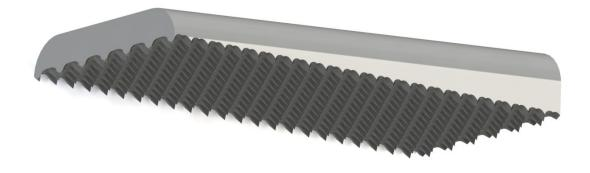
Figure 34 - Split Hopkinson pressure bar modified grip wedge.
