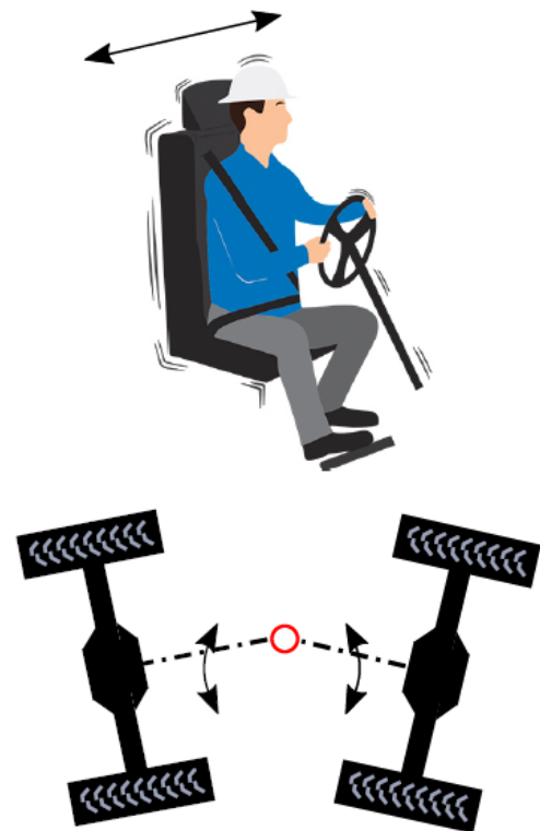
FIGURE 1: Yaw motion of an articulated frame steering vehicle during steering manoeuvres, resulting in lateral movement of operator.
