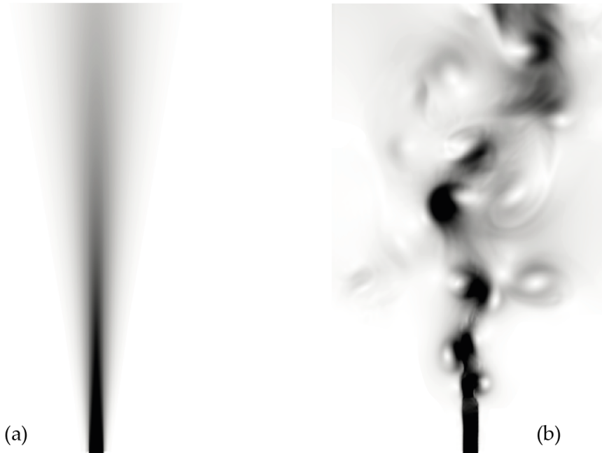
Fig. 2.10: Velocity field for a simulation of a jet using a RANS turbulence model in Fig. 2.10a and a LES turbulence model in Fig. 2.10b. The RANS model considers only the mean velocity whereas the largest velocity fluctuations are resolved in the LES model.
