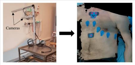
**Figure 6.** Two digital cameras (black arrows) were used to obtain the 3D photography of the thorax (left). Photography of the thorax documenting the ECG electrode positions (right).
