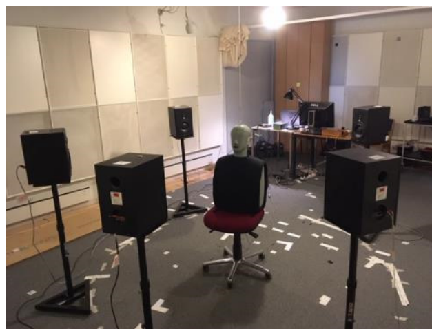
Figure 3. Picture of the test setup used for performing the SNR improvement measurements.
