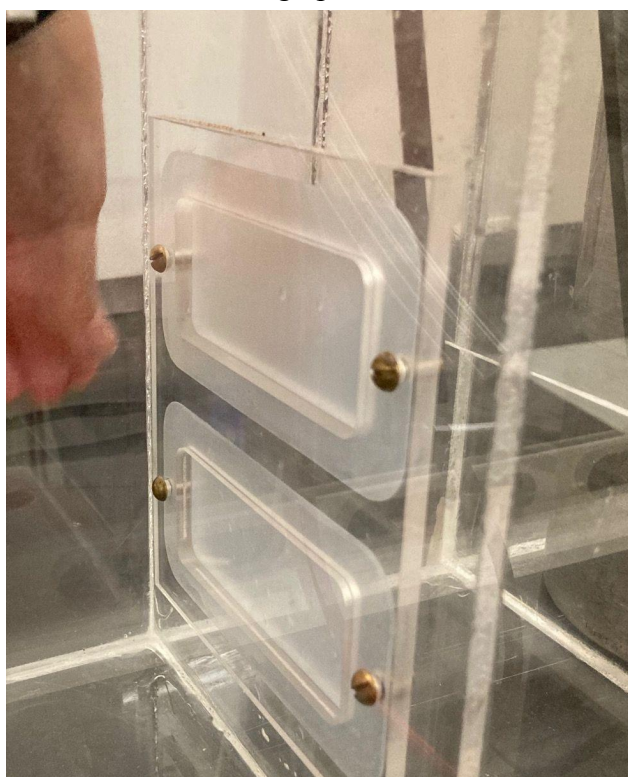
Figure 22: Architecture to hold osmotic membranes
