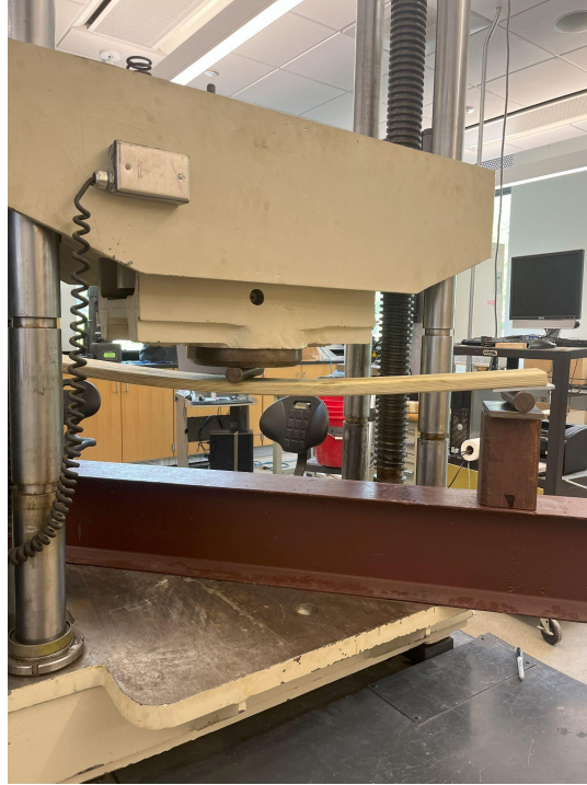
Figure 11. Experimental testing setup on the UTM; four-foot length 2x4” decking board mounted with two supports and load applied at the center.
