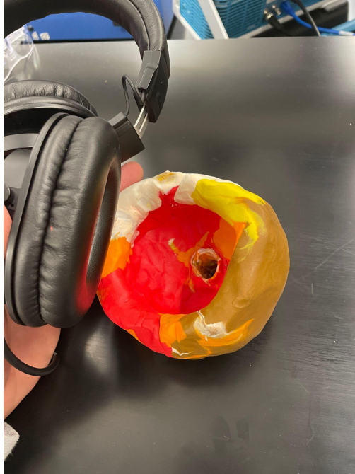
Figure 8 - A molded “ear” used in testing
