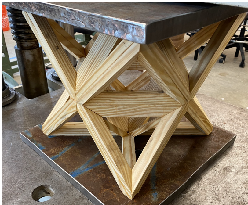
Figure 26: Truss between metal plates before the compression test started.
