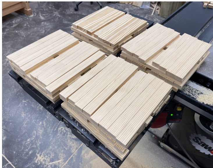
Figure 11: Image of wood members, measuring 0.5"x1"x8.5", stacked on each other.
