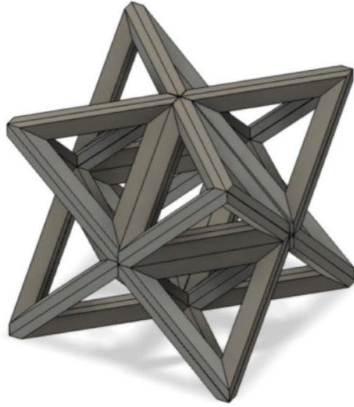
Figure 10: Eight pyramids are joined together to create a completed octet truss.
