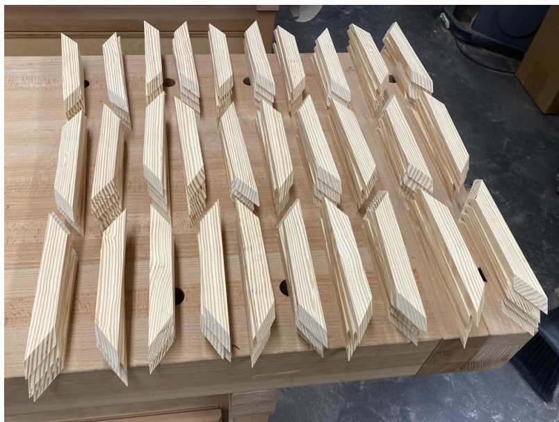
Figure 16: Image of wood members, after the faces have been cut, stacked on each other.
