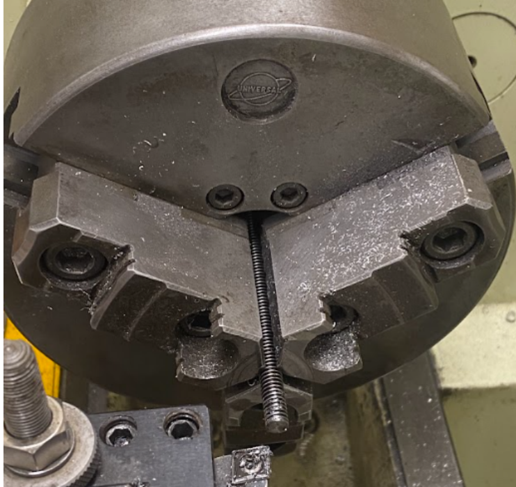
Figure 17: Machining Lead Screw with Lathe
