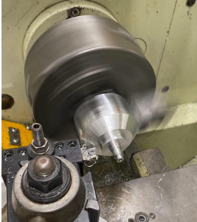
Figure 10: Machining Large Nozzle Using Lathe
