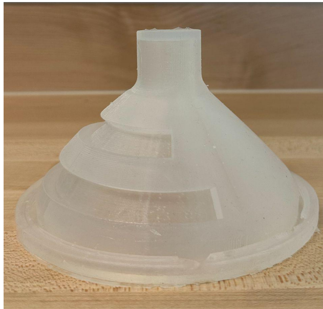
Figure 4.6: Flange Iteration 3 made out of Ecoflex 00-45.
