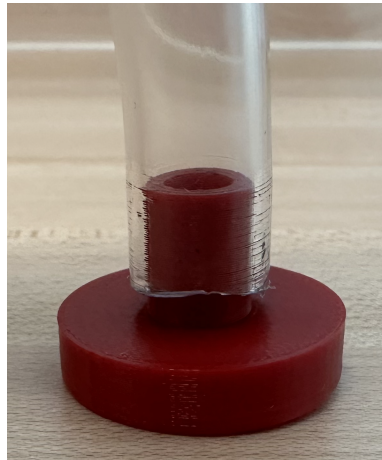
Figure 5.13: 3D printed part used to test applied vacuum pressure.
