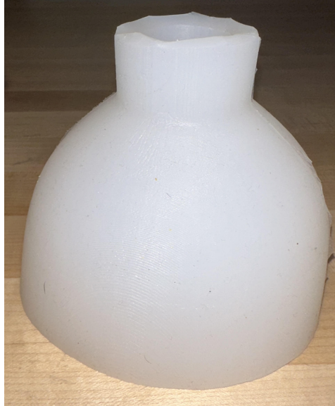
Figure 4.1: Flange Iteration 1 made out of Ecoflex 00-50.
