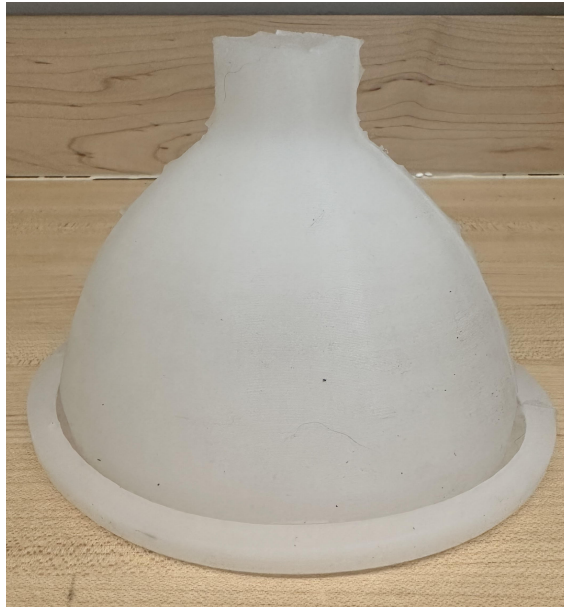
Figure 4.4: Flange Iteration 2 made out of Ecoflex 00-50.
