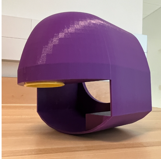
Figure 6.3: 3D single PLA print of housing design showing the outer facing bottle connection and accessibility opening.
