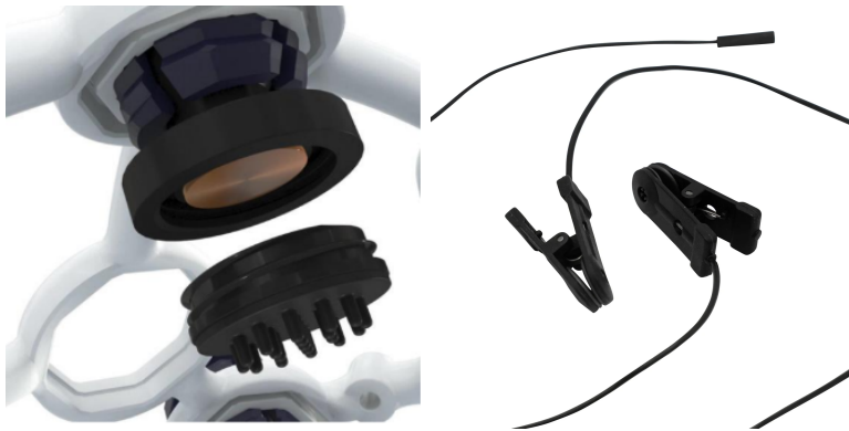
Figure 2.2: OpenBCI Shop Components. Cyton Amplifier (Top), Thinkpulse electrodes (Left), Grounding Ear Clips Electrodes (Right)
