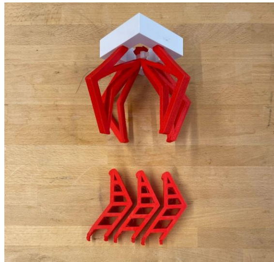
Figure 3.5: Flexible, 3-D printed fingers made with Prusa filament
