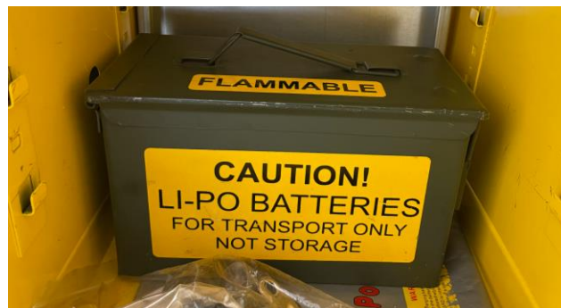
Figure 8.1: LiPo battery properly stored in multiple fire-safe containers
