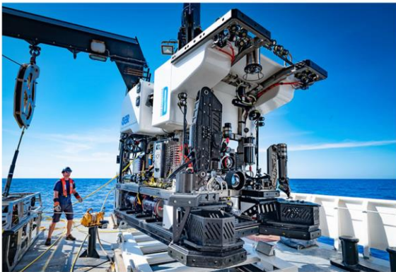
The remotely operated vehicle, Deep Discoverer , being recovered after completing 19 dives during the Windows to the Deep 2019 expedition. Image courtesy of Art Howard, Global Foundation for Ocean Exploration, Windows to the Deep 2019
