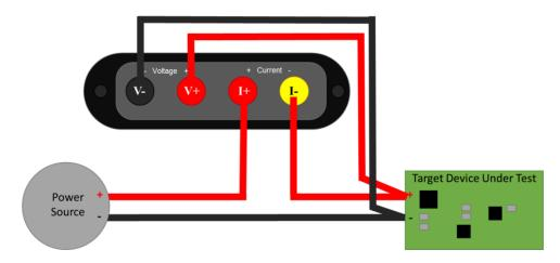
Figure 9. Power Measurement Setup
