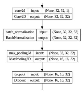
Figure 3: Convolutional layer block
