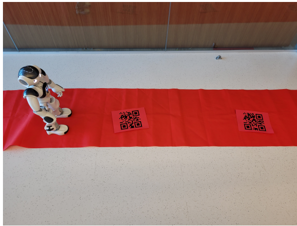
Figure 12: Demonstration Setup of the Nao robot with a straight path and 3 QR Codes
