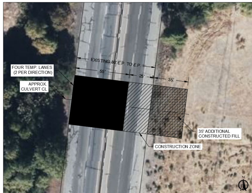
PHASE 1 - TRAFFIC ON THE WEST SIDE OF HWY 17, CONSTRUCTION ON EAST WITH ADDITIONAL 35' FILL
