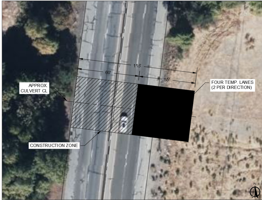
PHASE 2 - TRAFFIC ON THE EAST SIDE OF HWY 17, CONSTRUCTION ON WEST
