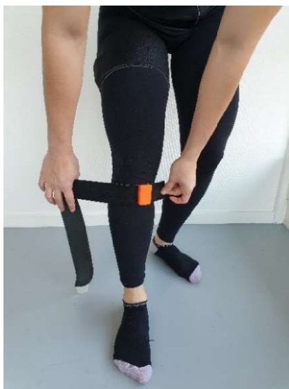
Figure 18: MTw Awinda right lower leg sensor placement flat on the shin bone (XSens Technologies, 2017).
