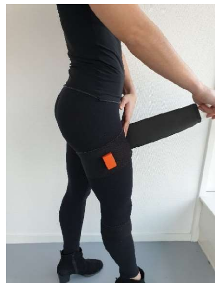
Figure 19: MTw Awinda right upper leg sensor placement on the lateral side above the knee (XSens Technologies, 2017).
