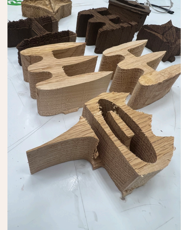
FIGURE 45 - Final CNC stamp pieces before sanding and polishing
