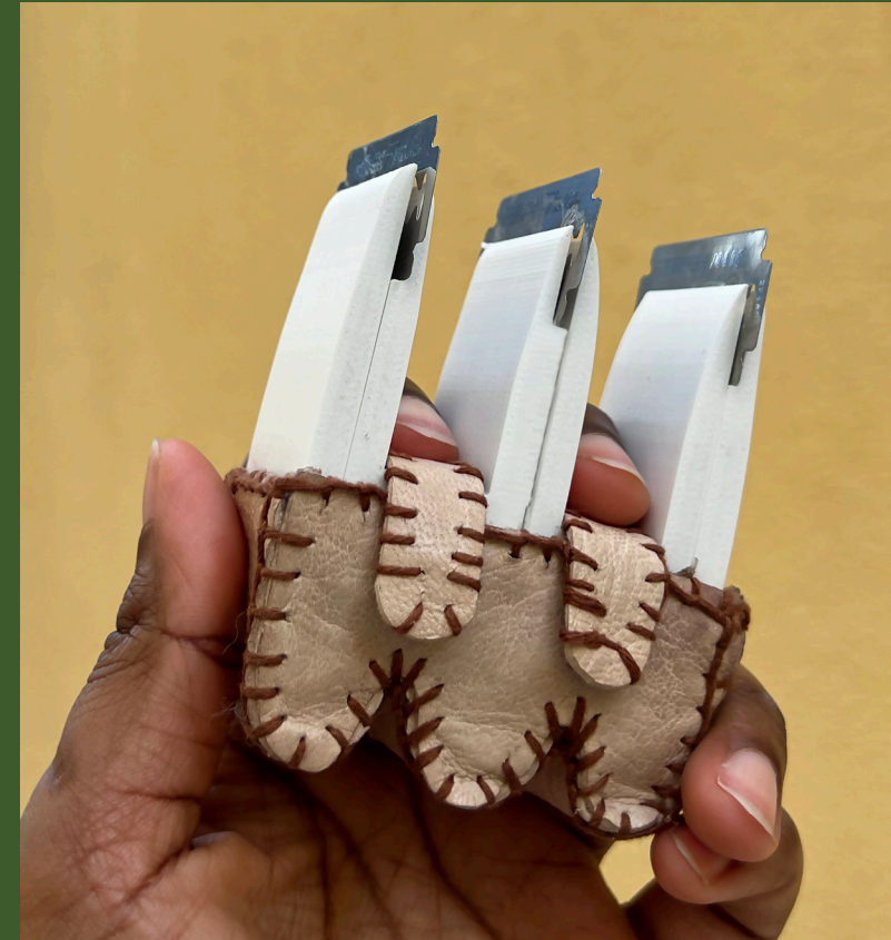
FIGURE 70 - FINAL OUTCOME Three strips blade holder side view (3D printed + leather)
