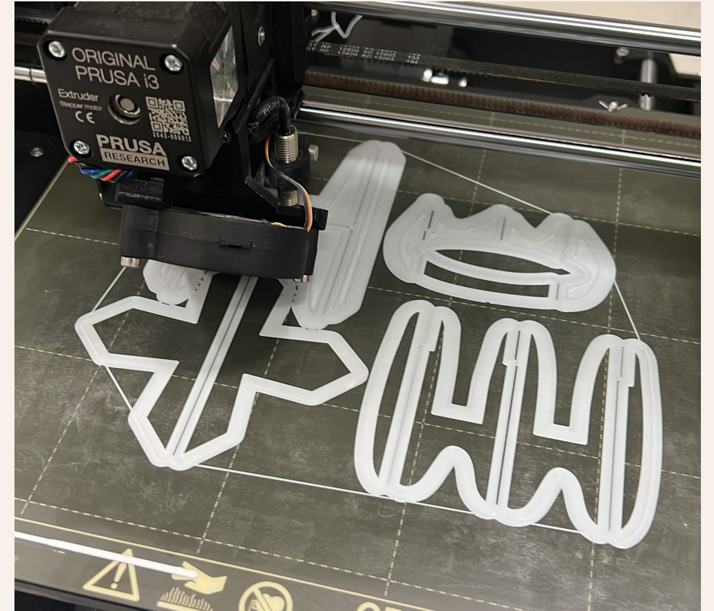
FIGURE 54 - 3D printing blade holders
