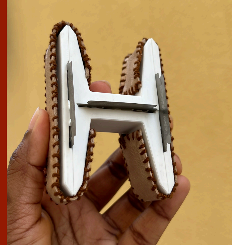
FIGURE 73 - FINAL OUTCOME H Blade holder side view (3D printed + leather)
