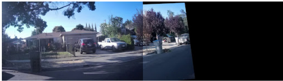
Figure 30: Image stitch from a homography matrix generated from regional keypoints
