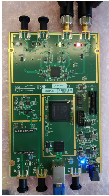
Figure 4.10: USRP B210 SDR transmitting and receiving radio signals, as indicated by the green and red LEDs, on the top right hand-side.
