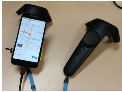
Figure 2.7: A Smartphone fixed onto a VR Controller [3]
