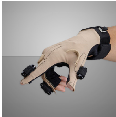
Figure 2.3: Hand tracking with data gloves from CyberTouch
