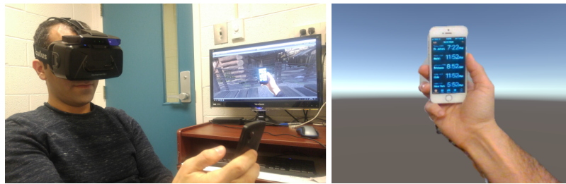
Figure 2.9: AV solution in Alae et al. [2]. On the left, is the setup with the RGB-Depth sensor. On the right, the user's hands and phone as rendered in the virtual environment.
