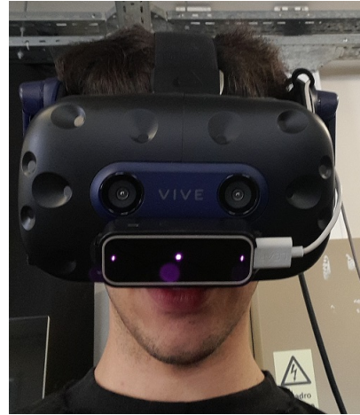
Figure 4.12: VR HMD with attached Leap Motion Controller
